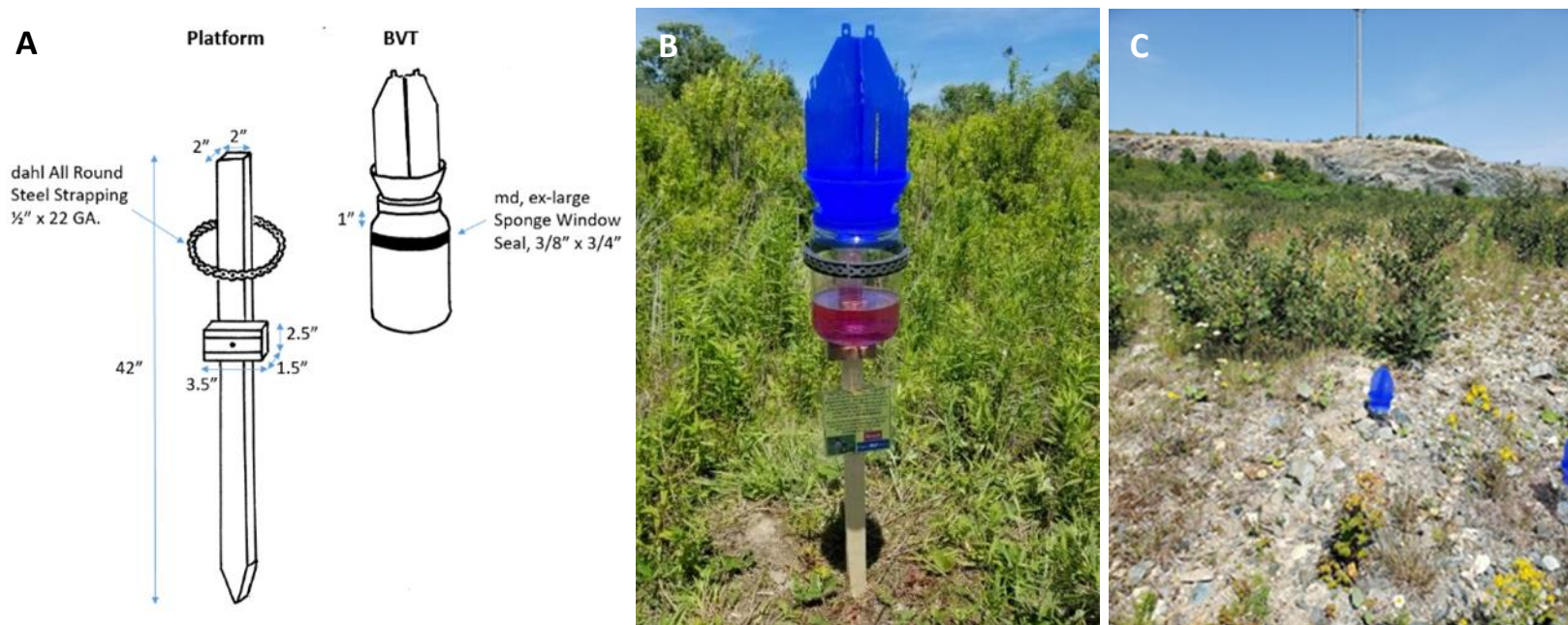
Figure 1.4: A depiction of the ways blue vane traps (BVTs) were installed in different regions. A) diagram of a BVT and platform used in the Carolinian Zone B) photograph of BVT set at Station Rd. site, in the Carolinian Zone dated 17 June 2021 C) photograph of BVT set into the ground at TGP site, in the Boreal Shield Ecozone, dated 19 July 2021 (provided by Dr. Carolyn Parsons). When not actively surveying at sites in the Carolinian Zone, BVTs and steel strapping were removed, while wooden stakes remained in place all field season.
