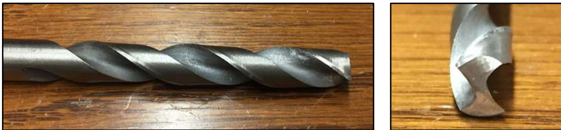
Figure 3.2. Drill bit used to modify microtiter plate wells
